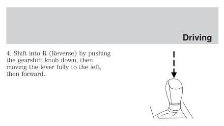
**Note:** The gearshift lever can only be moved to R (Reverse) by pushing the knob down before shifting to reverse. This is a lockout feature which protects the transmission from accidentally engaging R (Reverse) when intending to select 1 (First).
